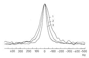
Fig. 4. <sup>17</sup>O-NMR spectra of distilled water. The half peak width of 138 Hz under no treatment (1) was reduced to 78 Hz (57% of the control) and 48 Hz (35%) after 20-min (2) and 4 days (3) of exposure, respectively, to far-infrared rays
