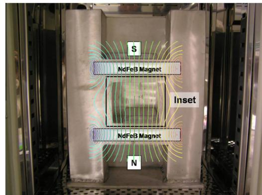
**Fig. A1.** Description of the SMF treatment device. The device used to treat cells with 0.23–0.28 T static magnetic fields is shown above along with field orientation and strength. <<http://www.biomedcentral.com/content/supplementary/1471-2164-10-356-S2.ppt>>.
